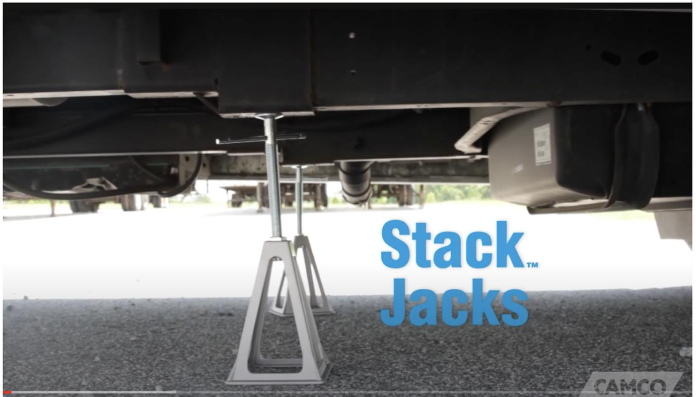
They are **not** strong enough to support the weight of the trailer, so don't jack them so far that they are pushing the trailer up in the air. They are only intended to keep the trailer from tipping back when people walk to the back, and to keep the trailer from rocking back and forth.
